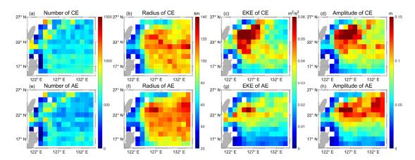
**Figure 4.** Distributions of eddy number (**a**,**e**), radius (**b**,**f**), the EKE (**c**,**g**), and amplitude (**d**,**h**). Values in each panel are averaged within  $1^{\circ} \times 1^{\circ}$  grid boxes where the eddy tracks snapshot are located. The boxes whose average depth is less than 300 m are masked to avoid unrealistic values. Upper panels show the distributions of cyclonic eddies (CEs), whereas lower panels show those of anticyclonic eddies (AEs).
