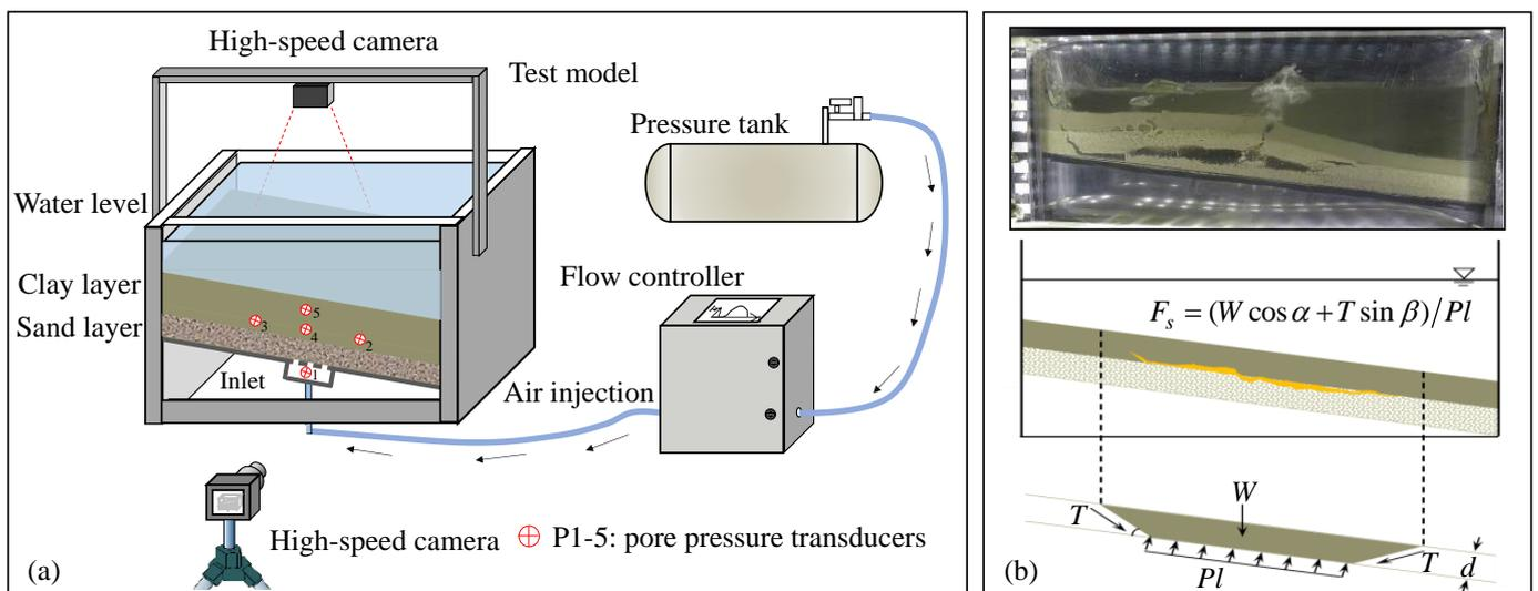
**Figure 5.** Investigation of submarine landslide induced by hydrate dissociation. (a) Schematic diagram of the experimental device; (b) Mode of submarine landslide induced by hydrate dissociation. Modified from [45].
