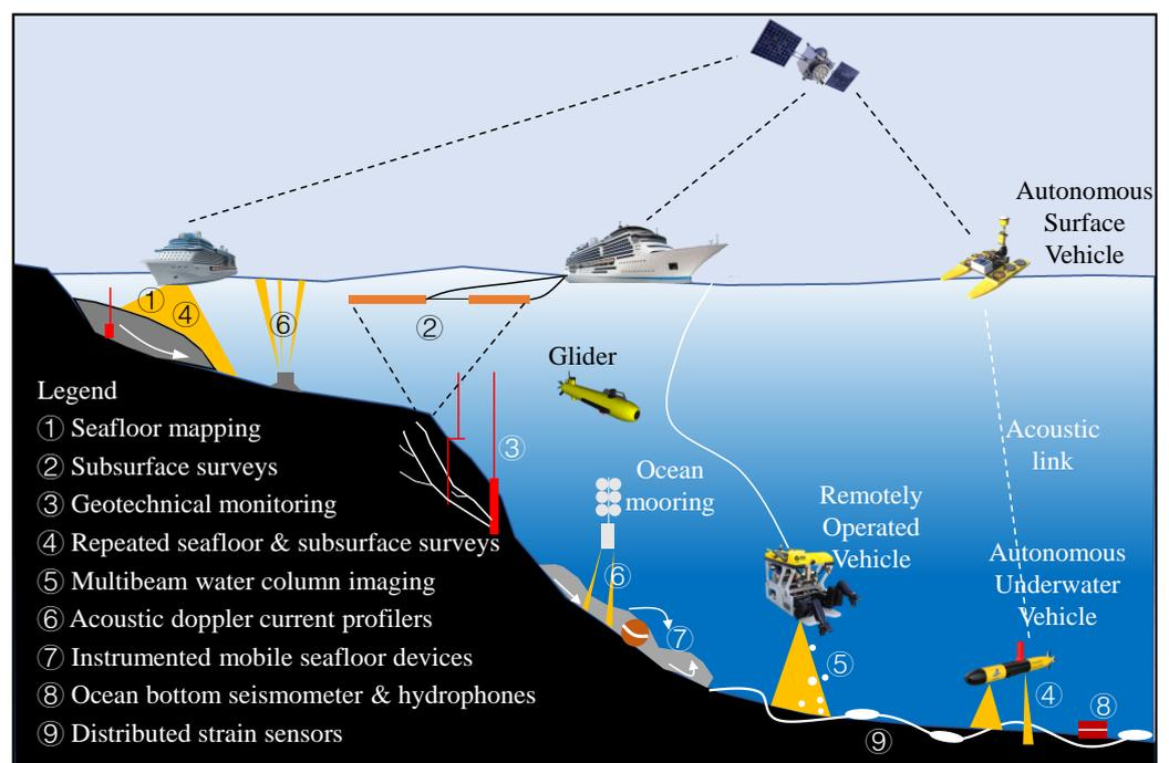
Figure 4. Conventional and emerging geophysical tools for submarine landslide in-situ investigations. Modified from [23].
