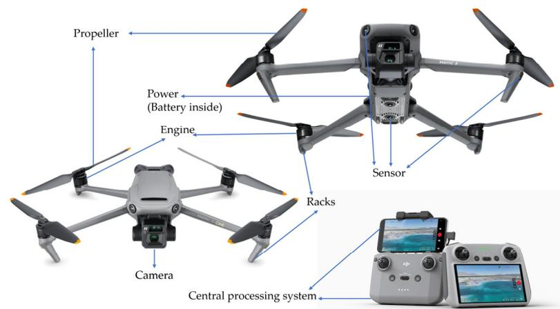
**Figure 1.** Structure of Drones.
