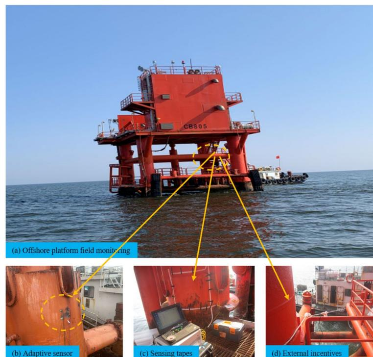
**Figure 19.** Field application of sensors.
