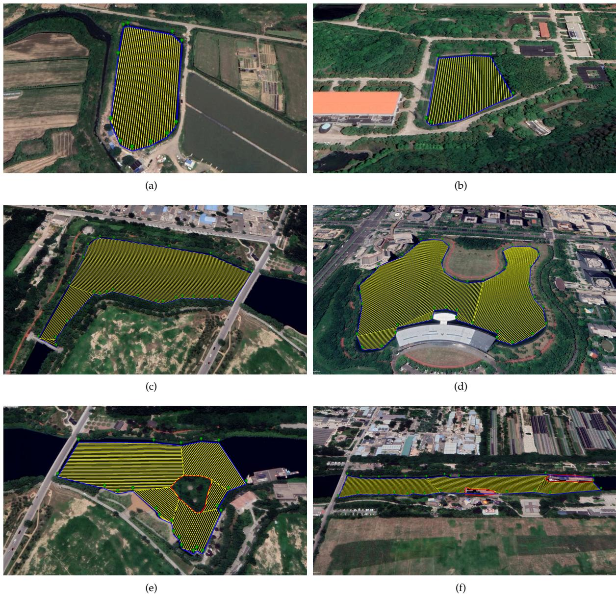
**Figure 9.** Result of WSCPP in different kinds of regions. The blue lines and the green points mark the region border. The red lines mark the obstacles border. The yellow lines mark the generated coverage path.
