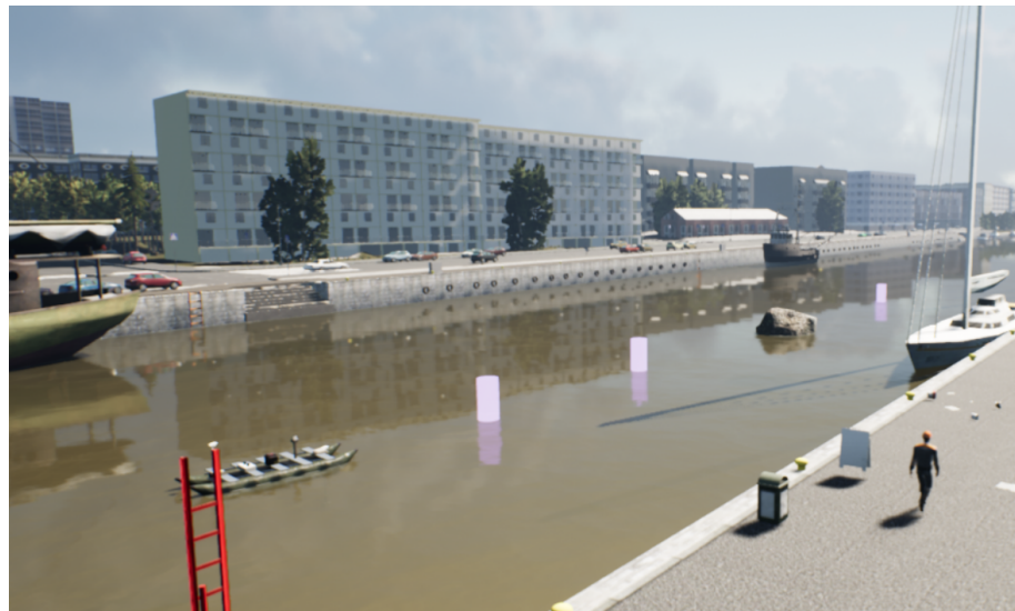
Figure 6. DRL model training setup in AILiveSim. The pink cylinders represent the global static waypoints while the rock is an obstacle amidst the planned trajectory. Note that the static waypoints are not recomputed when an obstacle is encountered.
