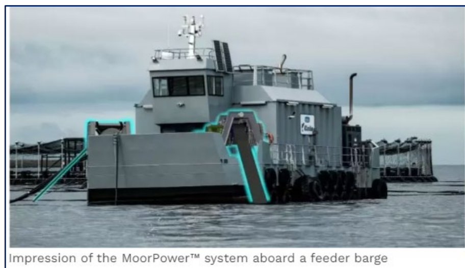
Figure 27. Moorpower™ floating feed barge showing wave energy converters in green—image from https://blueeconomyrc.com.au/project/moorpower-scaled-demonstrator/ (accessed on 22 September 2022).
