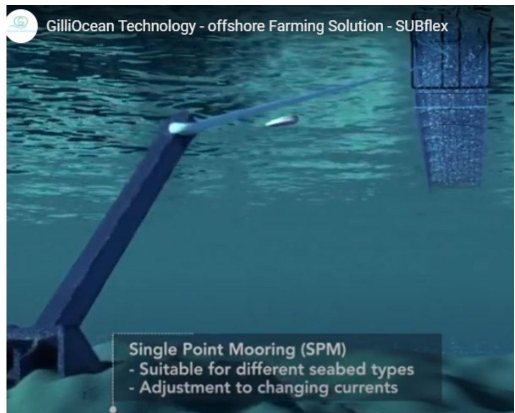
Figure 12. Linear tensile system—single point mooring—Gili SUBFlex — ( https://www.giliocean.com/selected-projects (accessed on 22 September 2022)).
