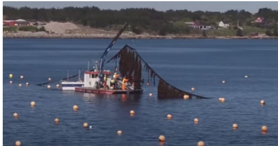
Figure 16. Crane manipulating longline with hand-over-hand harvesting—image from https://seaweedsolutions.com/ (accessed on 22 September 2022).
