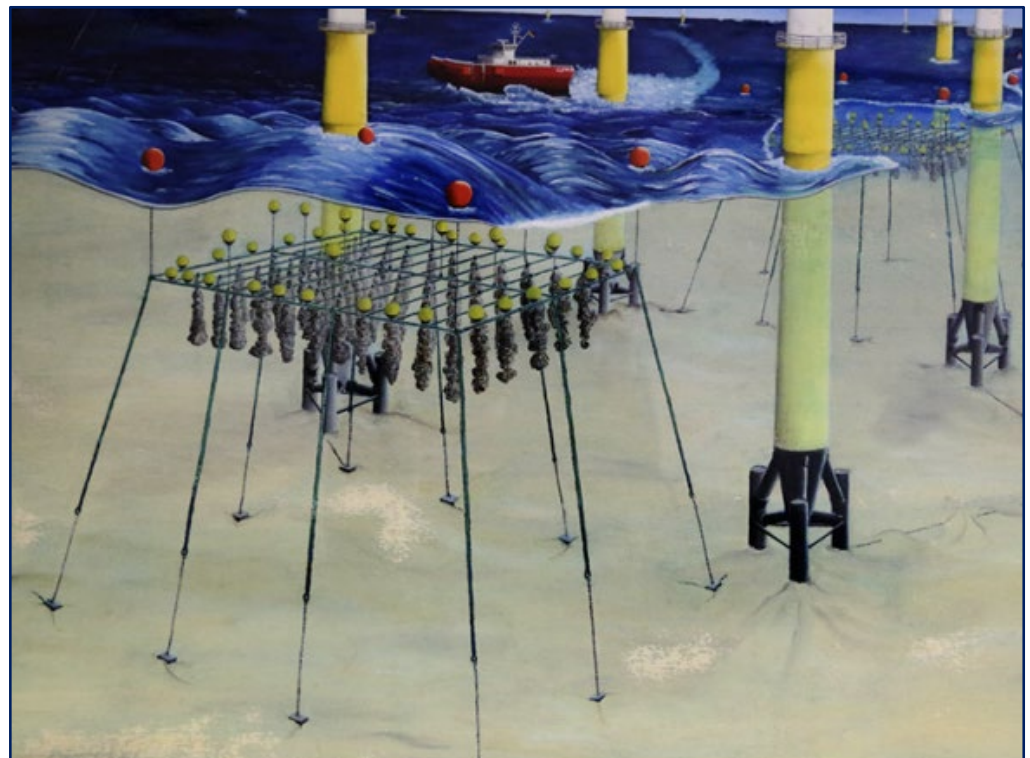
Figure 25. Cable tethered seaweed/IMTA-tensile system in offshore wind park [13].
