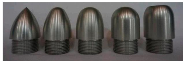
Figure 3. Five head shapes. The hemispherical angles from left to right are  $0^\circ$ ,  $57^\circ$ ,  $70^\circ$ ,  $90^\circ$ ,  $180^\circ$ .
