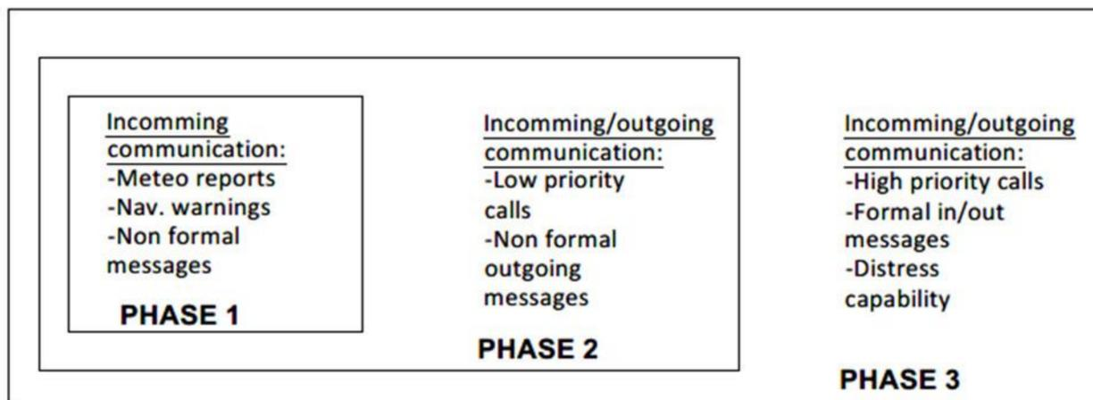
**Figure 8.** Development phases of SDR for the needs of maritime communications.
