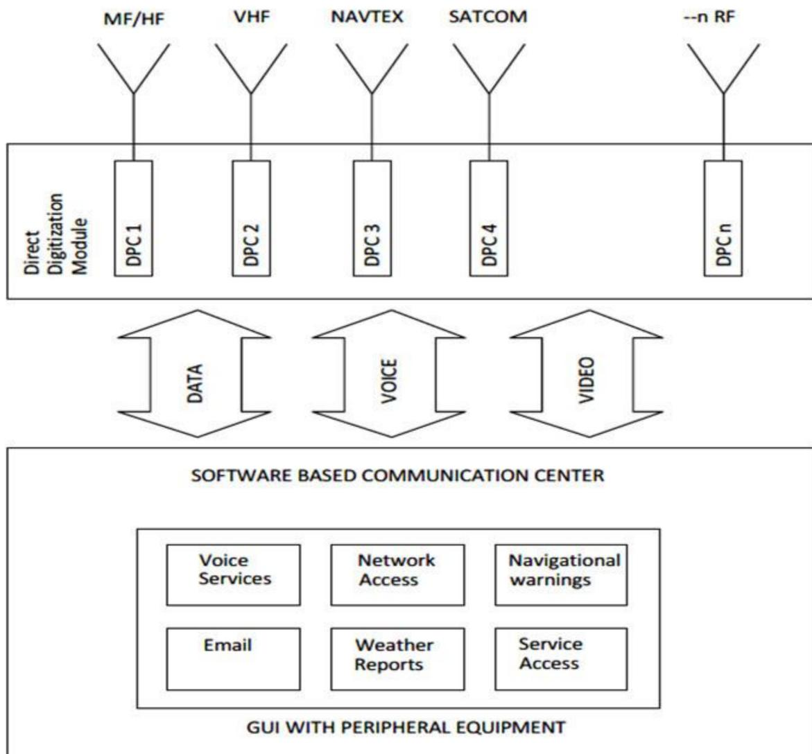
**Figure 7.** Model of the maritime communications system based on the SDR approach.
