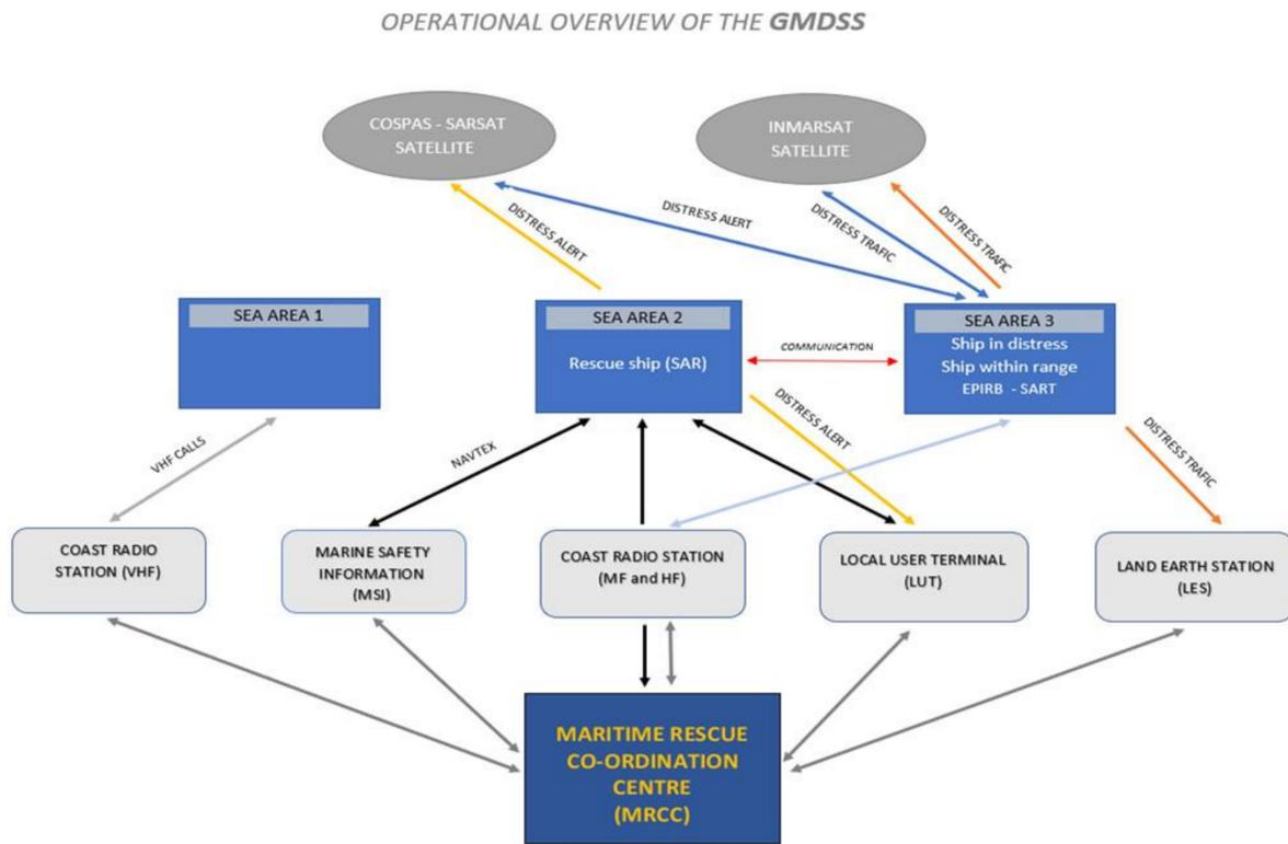
Figure 1. GMDSS communication used on a ship.
