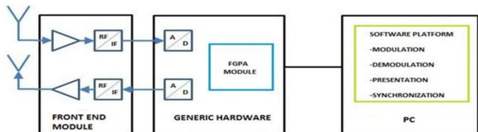
Figure 4. A generic hardware configuration of SDR.
