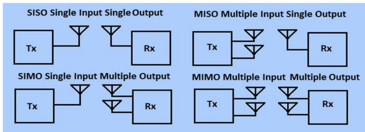
Figure 6. Types of MIMO approaches in the design of the antenna.
