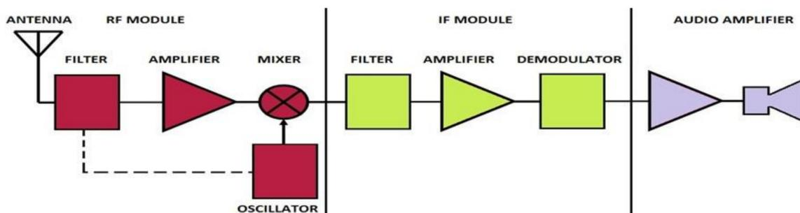
Figure 2. Block scheme of a typical radio receiver.
