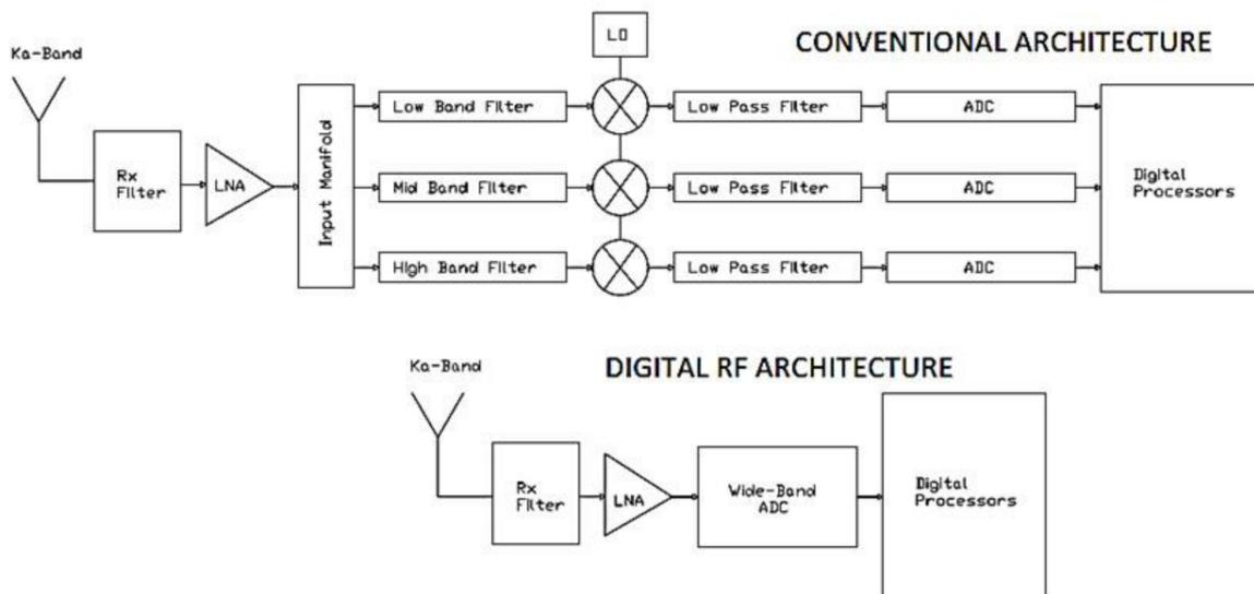
**Figure 5.** Comparison of conventional and digital RF architecture.
