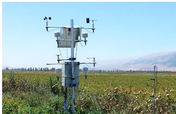
Figure 2. Bowen ratio station (NESA) installed in the potato field.
