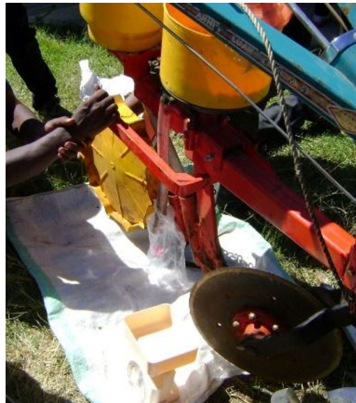
Figure 2. Calibration of a single-row no-till planter. The drive wheel is turned by hand and the seeds collected in a plastic bag attached to the seed outlet. Seeds can be counted and/or weighed to calculate seeding rates per ha.
