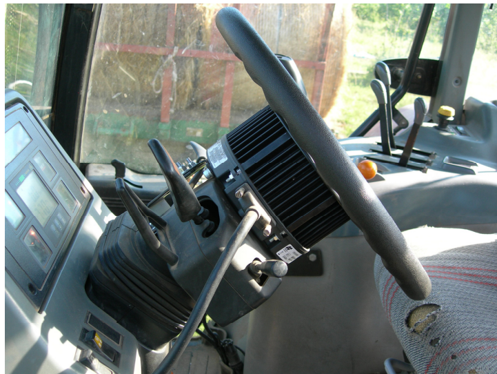
Figure 1. Steering wheel with automatic guidance device.
