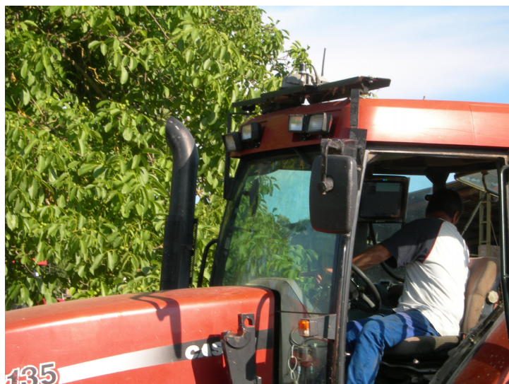
Figure 2. Monitor and antenna installed on the tractor.
