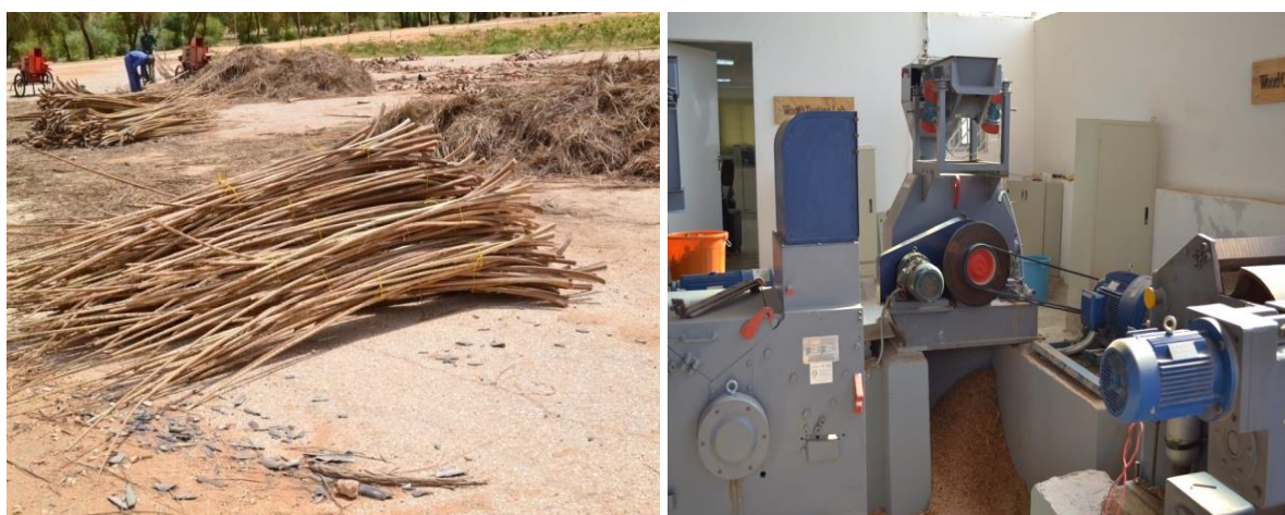
Figure 1. Date palm fronds without leaflets and the ring flaker machine (BX-466).
