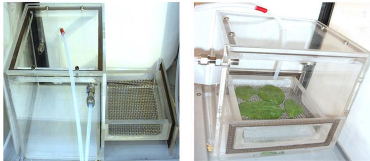
**Figure 10.** Modified ozone fumigation system.
