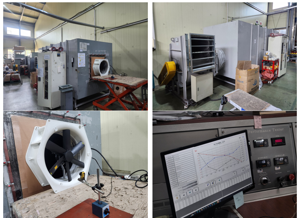
Figure 5. Greenhouse circulation fan performance testing laboratory (variable supply device, flow straightening grid, settling chamber).
