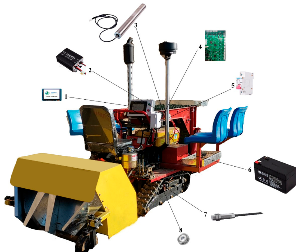
Figure 2. Schematic diagram of the whole machine structure. (1) Human–computer interaction touch screen; (2) Power converter; (3) DC drum motor; (4) The main controller; (5) Air switch; (6) Power supply; (7) Hall sensor; (8) Speed gear.
