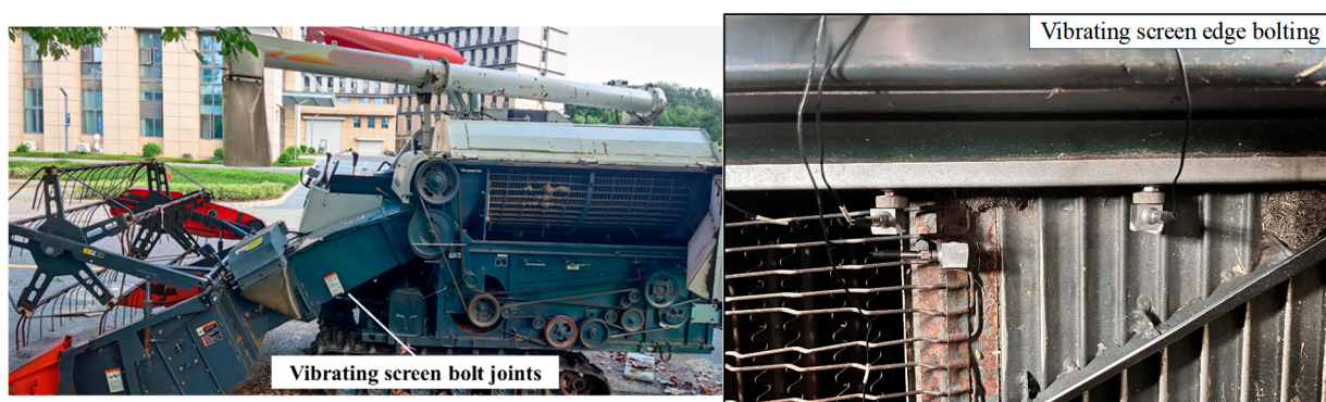
Figure 9. Distribution of vibrating screen bolt measurement points.
