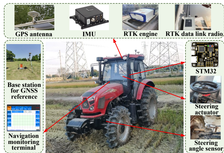
Figure 3. The main composition of the autonomous navigation system for wheeled tractor.
