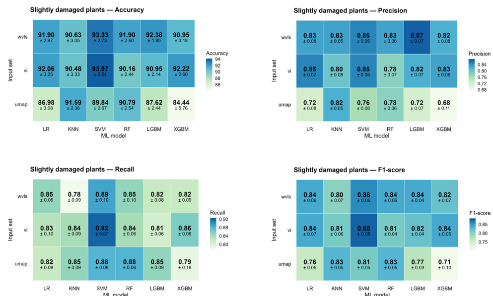
Figure 8. Classifier performance at the early-detection threshold (slightly damaged plants) across spectral inputs (wvls, VI, UMAP) using 10-fold nested cross validation; Accuracy, Precision, Recall, F1-score (mean ± SD).
