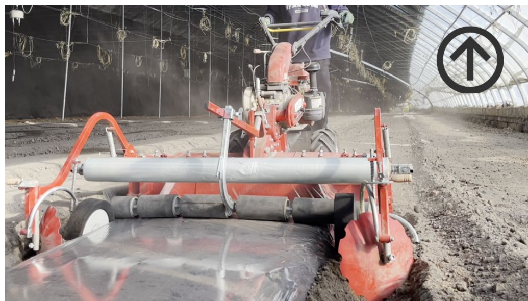
Figure 16. Field testing of the ridge-mulching machine. The arrow indicates the forward direction of the machine.
