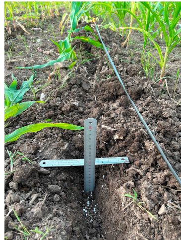
Figure 13. Field measurement of topdressing depth.
