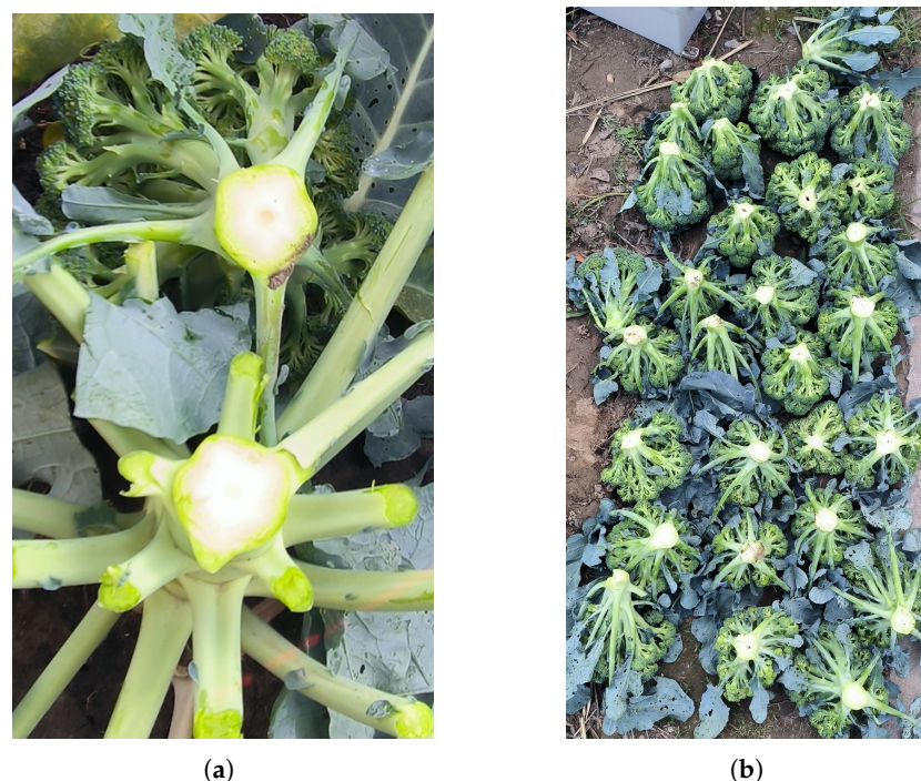
Figure 15. Photos about the cutting quality in the field test: (a) Cross-section of the stem of a single broccoli specimen; (b) Harvested broccoli specimens after cutting by the end effector.
