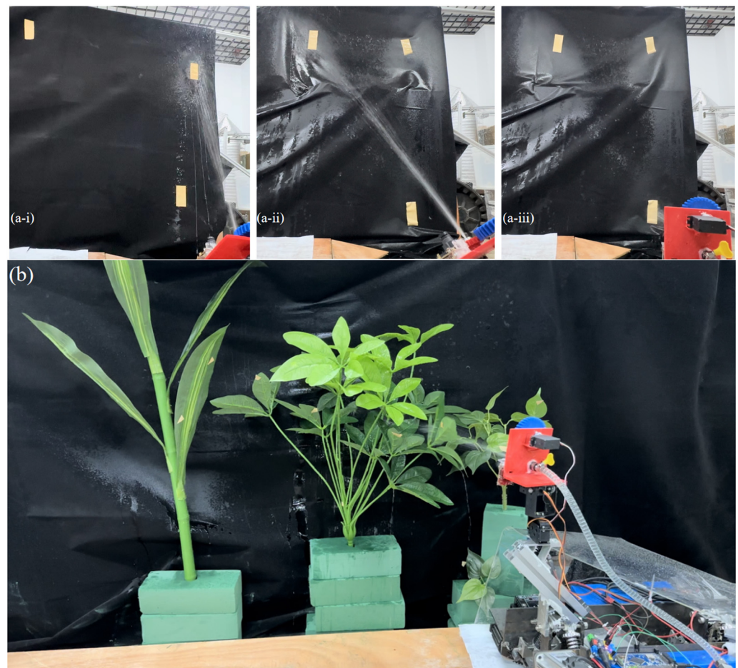
Figure 19. The real-life spraying tests. Sub-image (a) shows the nozzle's adjustment of spray parameters; (b) is a screenshot of the actual spraying.
