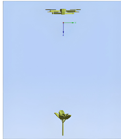
Figure 10. Seedling-stage rapeseed-downwash air flow fluid-structure interaction simulation model.
