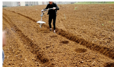
(a) Prototype test of hole-forming machine.
