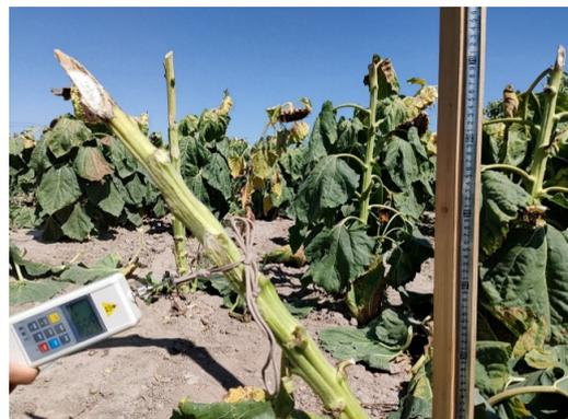
**Figure 6.** Measurement of the critical bending angle of sunflower stalks.
