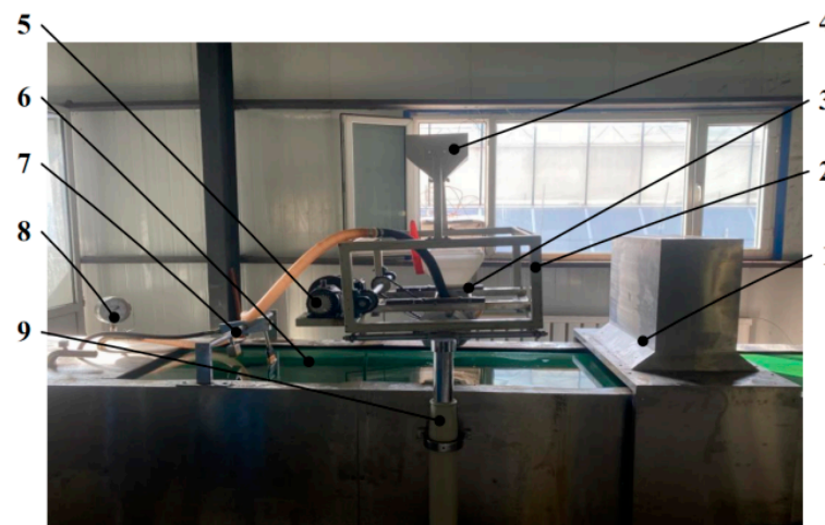
Figure 6. Test bench structure schematic. 1. Monitoring device; 2. Fixed bracket; 3. Seed-metering device; 4. Seed box; 5. Motor; 6. Belt; 7. Oil circuit system; 8. Wind system; 9. Altitude adjustment device.
