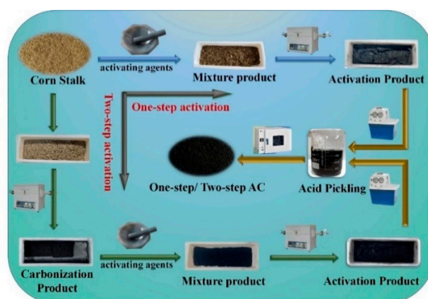
Figure 1. Experimental flowcharts for one-step and two-step preparation of AC.
