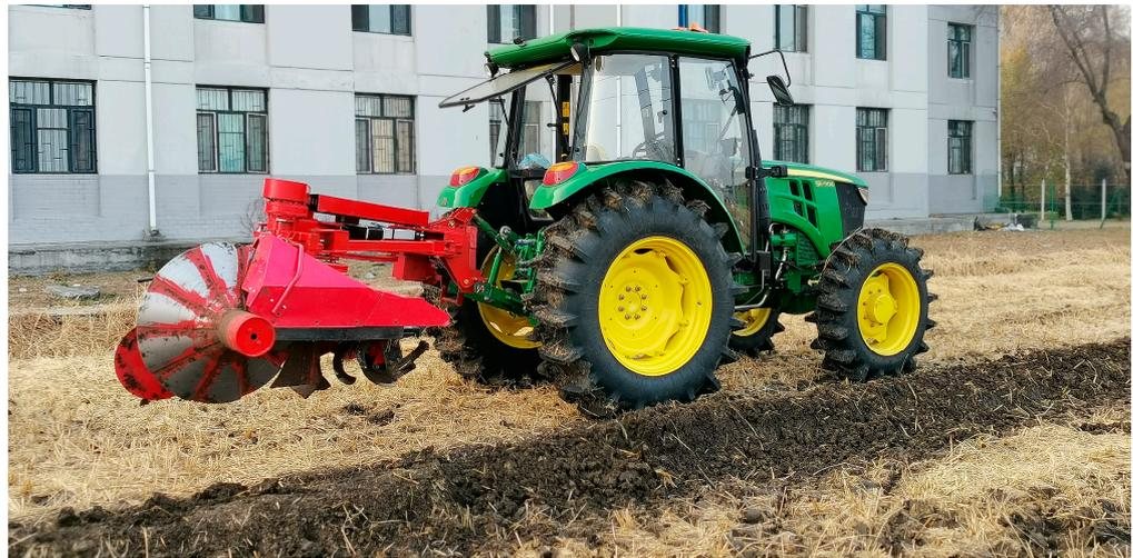
**Figure 10.** The operational effect of rotary-cutting soil collection device in paddy field.
