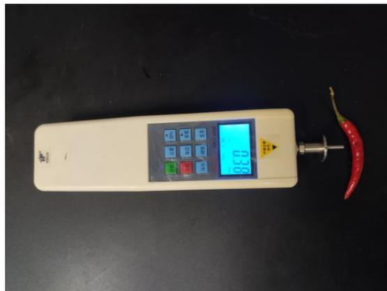
Figure 6. GY-4 digital hardness tester.
