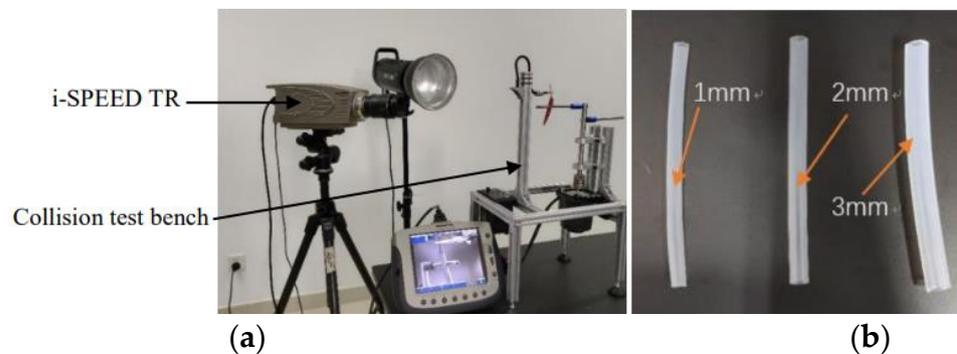
**Figure 5.** Pilgrim's collision velocimetry equipment (a) and flexible hoses of different thicknesses (b).
