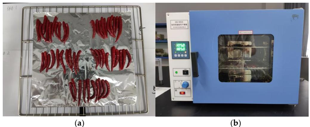
**Figure 4.** An experiment to measure the water content of peppers (a) in pods using a drying oven (b).
