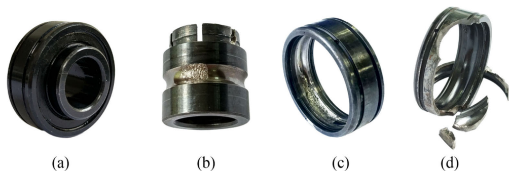
Figure 4. Photos of tested bearings: (a) Normal bearing; (b) Inner race wear; (c) Outer race wear; (d) Outer race fracture.
