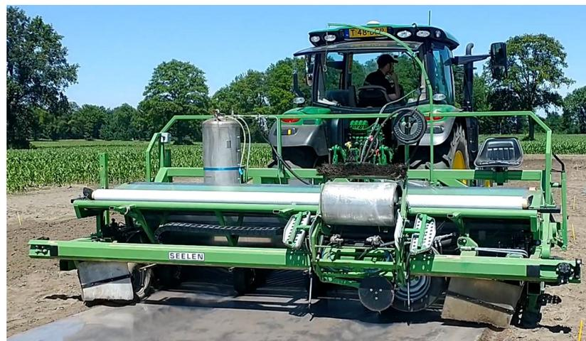
**Figure 1.** Machine for automatic tarping.
