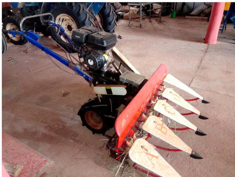
**Figure 6.** Mini grain reaper machine.
