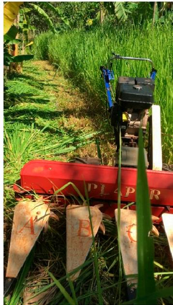
**Figure 11.** Deposition of cut grass leaves by GRM.
