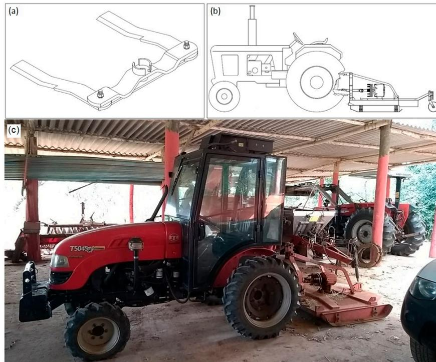
**Figure 5.** Tractor mounted rotary brushcutter: (a) rotating blades; (b) implement connected to the tractor's three-point system; (c) tractor and implement utilized.
