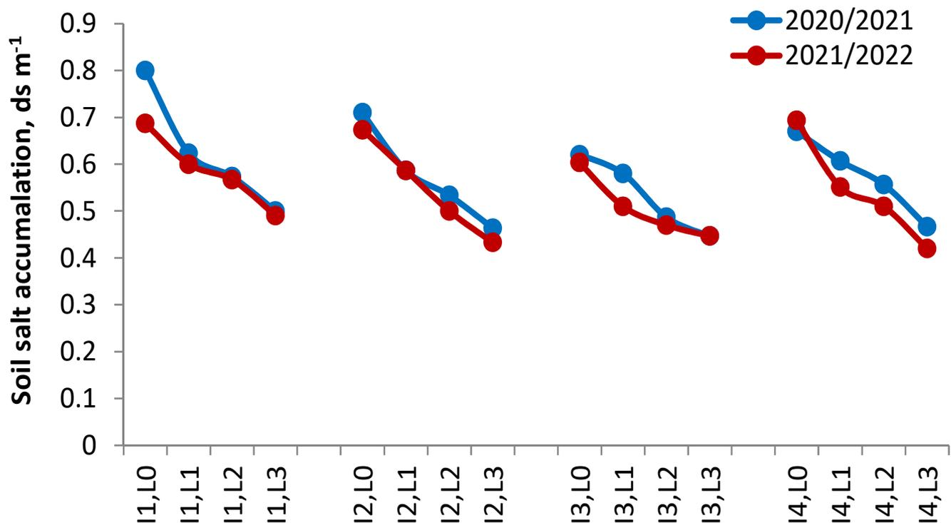
**Figure 8.** The performance of partial root-zone drying technique and soil organic mulch on salt accumulation in the root zone. I1, 100% full irrigation (FI); I2, 75% FI; I3, 50% FI; I4 (PRD), 50% FI; L0, zero organic soil mulch (control); L1, a single layer of organic soil mulch; L2, two layers of organic soil mulch; L3, three layers of organic soil mulch; PWP, permanent wilt point; FC, field capacity.
