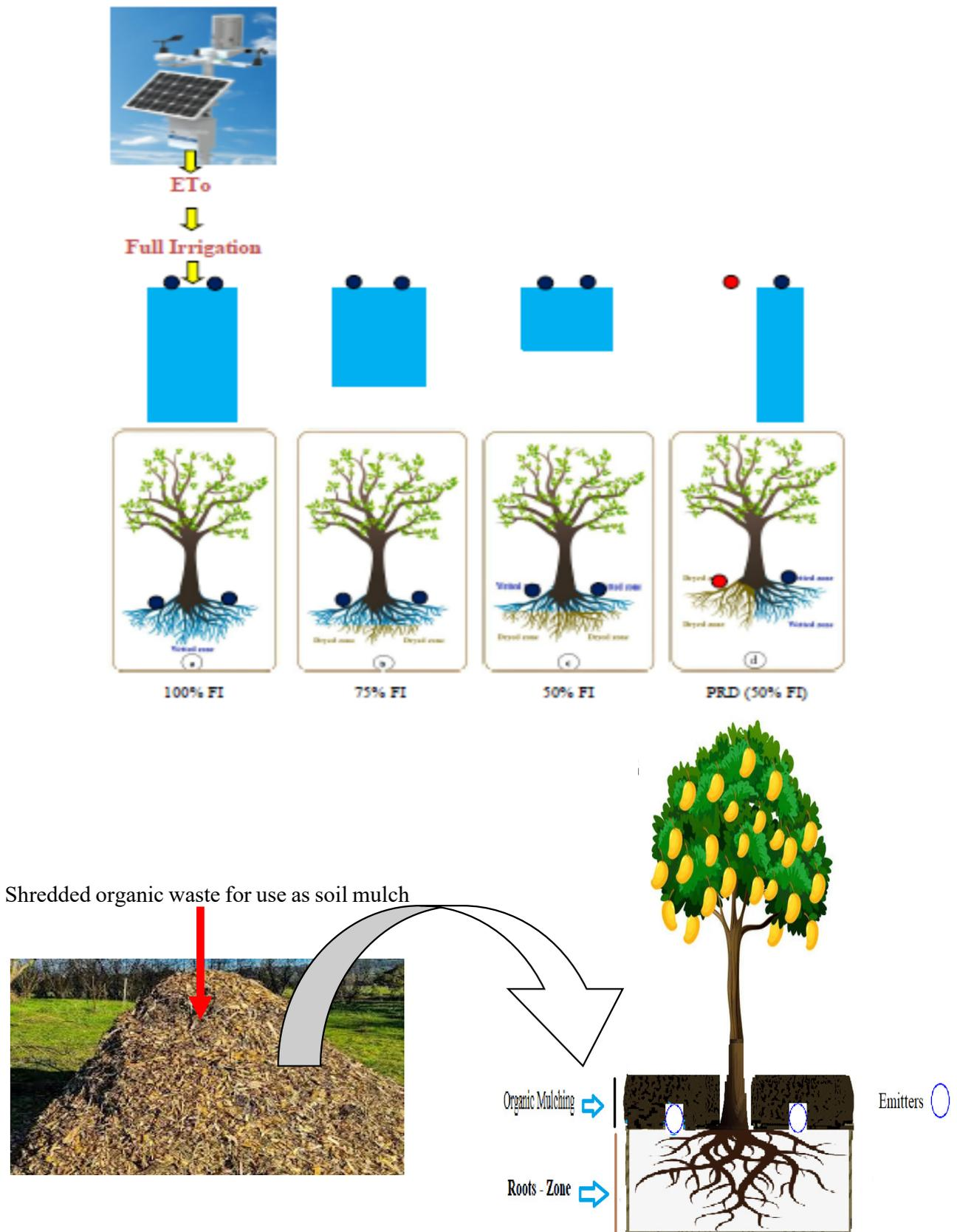
**Figure 1.** Distribution of main and sub-main factors according to experimental design. Main factor: Schematic of the irrigation pattern in 100% FI (a), 75% FI (b), 50% FI (c) and PRD (50%) (d). Sub-main factor: Organic mulching.
