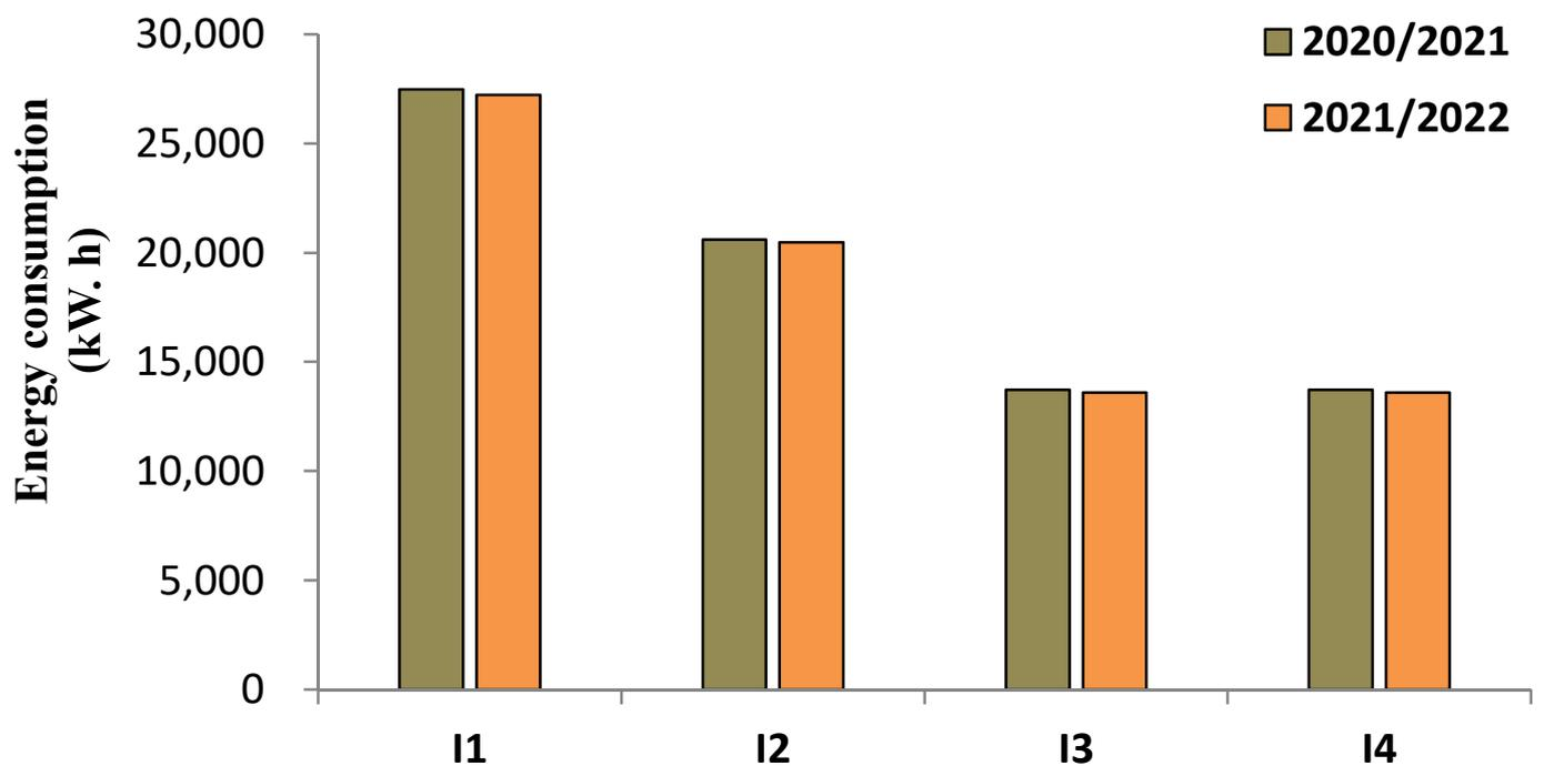
Figure 12. Energy consumed with scheduled deficit of irrigation. I1, 100% full irrigation (FI); I2, 75% FI; I3, 50% FI; I4 (PRD), 50% FI.
