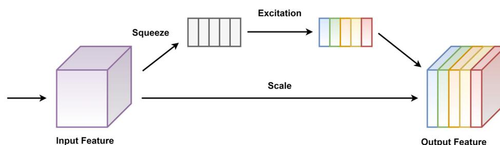
**Figure 10.** The overview of SE module.
