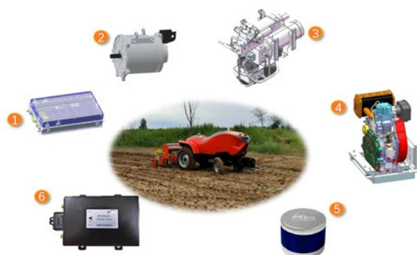
**Figure 23.** Test process and prototype demonstration: 1. Battery pack; 2. Motor; 3. Hydraulic station; 4. Range extender; 5. Laser radar; 6. Integrated inertial navigation.
