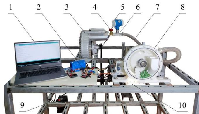
**Figure 10.** Platform of compensation device performance test. (1) Upper computer, (2) compensation control system, (3) fan, (4) regulating valve, (5) digital pressure gauge, (6) tee joint, (7) pipe, (8) large- and medium-sized grain crops compensation device, (9) frequency transformer, (10) performance monitoring system.
