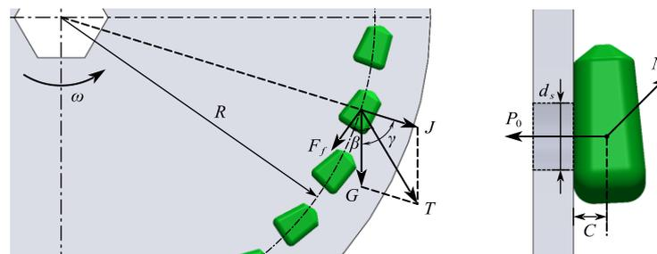
Figure 4. Force analysis diagram of the seed filling state.
