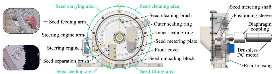
**Figure 1.** Overall structure of large- and medium-sized grain crop compensation device.
