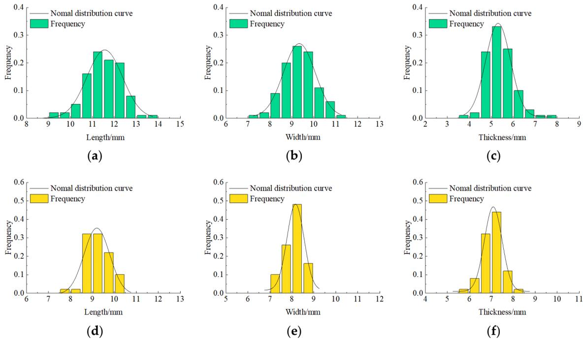
**Figure 3.** Normal distribution diagram of the three-axis dimensions of corn and soybean seeds: (a) corn length distribution, (b) corn width distribution, (c) corn thickness distribution, (d) soybean length distribution, (e) soybean width distribution, (f) soybean thickness distribution.
