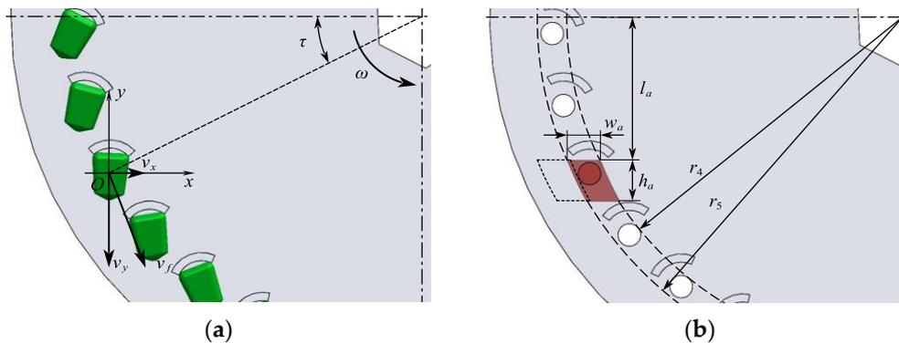
**Figure 7.** Motion analysis of seed feeding process and structural parameters of seed feeding arm: (a) motion analysis of seed seeding process, (b) structural parameters of seed feeding arm.
