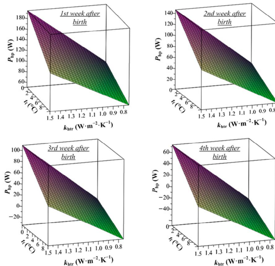
**Figure 1.** Required power capacity  $P_{hp}$  of floor-mounted heating panels depending on the floor temperature  $t_f$ , heat transfer coefficient  $k_{htr}$ , and age of pre-nursery pigs.
