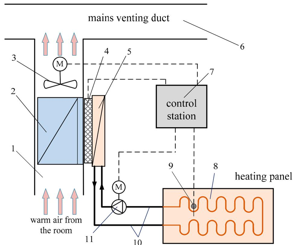
**Figure 2.** Block diagram of local floor-mounted heating installation for preweaning pigs with the application of thermoelectric effect: 1—duct of the cold air circuit; 2—air heat-exchanger at the cold side of Peltier elements; 3—electric fan; 4—Peltier elements; 5—water heat-exchanger at the hot side of Peltier elements; 6—mains venting duct; 7—control module; 8—floor-mounted heating panel; 9—temperature sensor; 10—duct of the hot air circuit; 11—circulation heat pump.
