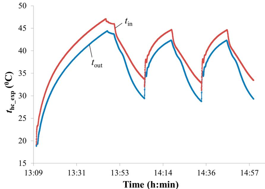
**Figure 5.** Temperature of the heat-carrier  $t_{hc\_exp}$  in the input into the panel  $t_{in}$  and in its output  $t_{out}$ .
