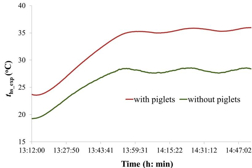
**Figure 6.** Surface temperature  $t_{hs\_exp}$  of the floor-mounted heating panel without animals and at 70% charging of the crate with pre-nursery pigs.
