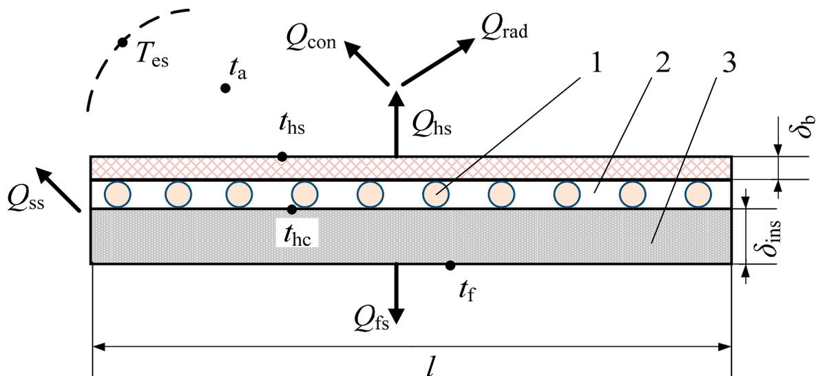
Figure 3. Diagram for calculating thermal capacity of the heating panel: 1—substrate; 2—heat-carrier; 3—thermal insulation.
