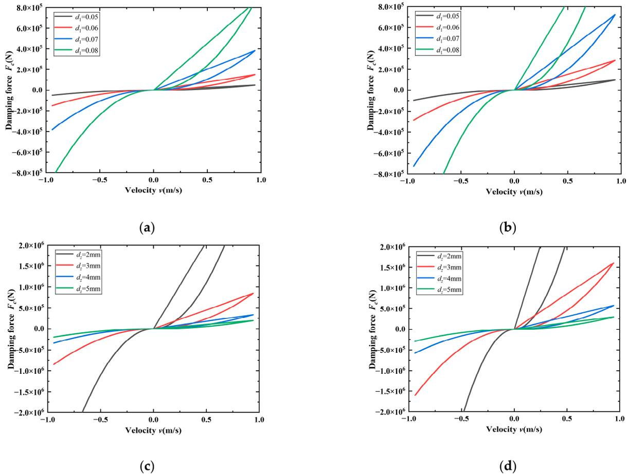
**Figure 9.** Variation in damping force with parameters: (a,b) are the changing trends of the damping force of traditional hydro-pneumatic suspension and 3-damping hole hydro-pneumatic suspension with the cylinder diameter of the hydraulic cylinder; (c,d) are the changing trends of damping force of traditional hydro-pneumatic suspension and 3-damping hole hydro-pneumatic suspension with damping aperture.
