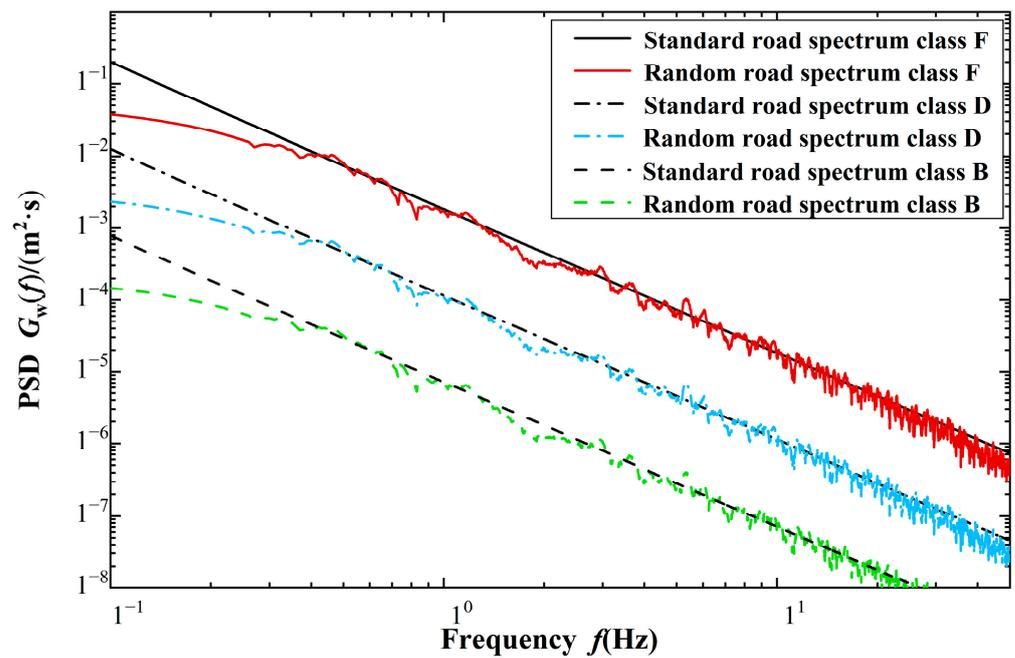
Figure 3. Comparison of PSD curve between random road and standard road.
