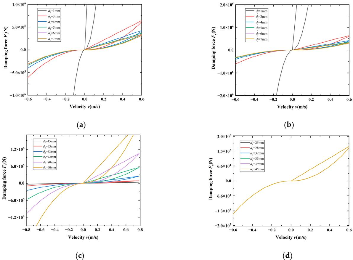
**Figure 8.** Relationship between damping force and parameters: (a) relationship with  $d_z$ , (b) relationship with  $d_j$ , (c) relationship with  $d_2$  and (d) relationship with  $d_1$ .
