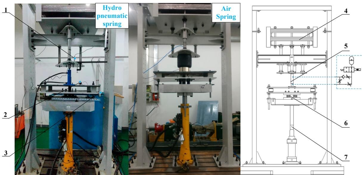
**Figure 11.** Vibration test bench based on air spring and hydro-pneumatic spring: (1) acceleration sensor, (2) displacement sensors, (3) displacement sensors, (4) steel plate, (5) hydraulic cylinder, (6) tire and (7) servo actuator.
