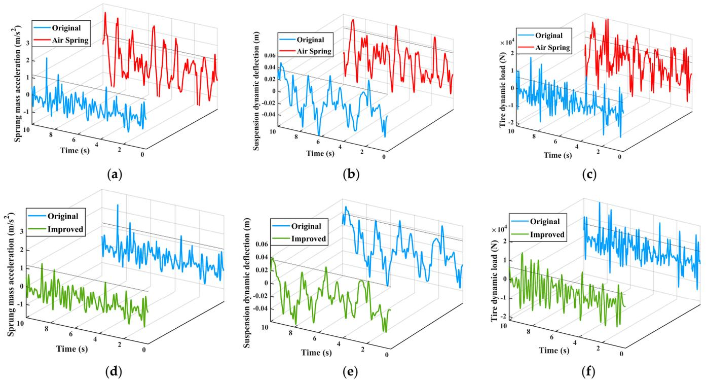
**Figure 17.** Comparison of test results of three kinds of suspension: (a–c) are the comparison between air suspension and original hydro-pneumatic suspension in terms of sprung mass acceleration, suspension dynamic deflection, and tire dynamic load, (d–f) are the comparison between the improved hydro-pneumatic suspension and the original hydro-pneumatic suspension in terms of sprung mass acceleration, suspension dynamic deflection, and tire dynamic load.
