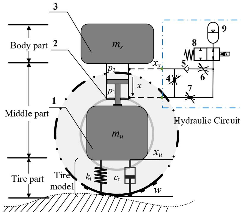
**Figure 2.** Quarter hydro-pneumatic suspension model: (1) unsprung mass, (2) hydraulic cylinder, (3) sprung mass, (4) damping hole, (5) check valve, (6) damping hole, (7) damping hole, (8) electromagnetic on-off valve and (9) accumulator.
