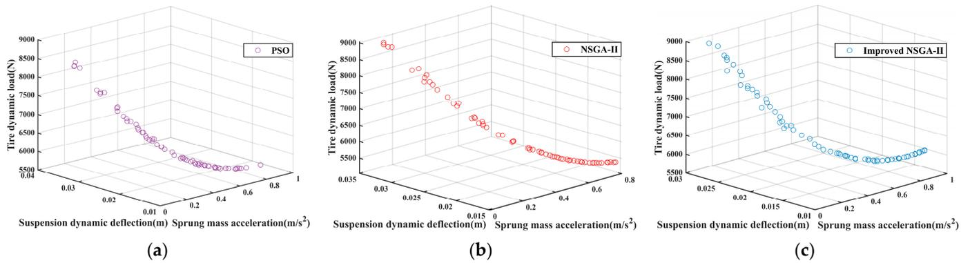
**Figure 14.** Comparison of Pareto fronts of PSO, NSGA-II and improved NSGA-II: (a) is the Pareto fronts of the PSO algorithm, (b) is the Pareto fronts of the NSGA-II algorithm, (c) is the Pareto fronts of the improved NSGA-II algorithm.
