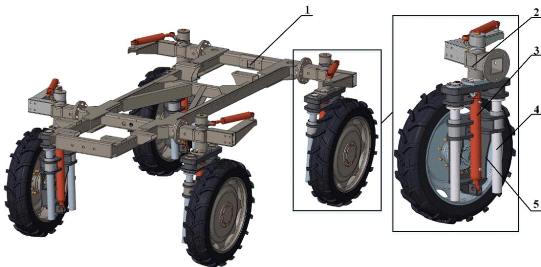
**Figure 1.** Design of sprayer hydro-pneumatic suspension chassis: (1) the frame, (2) the steering system, (3) the hydro-pneumatic suspension hydraulic cylinder, (4) the guide mechanism and (5) connecting housing of hydro-pneumatic suspension.
