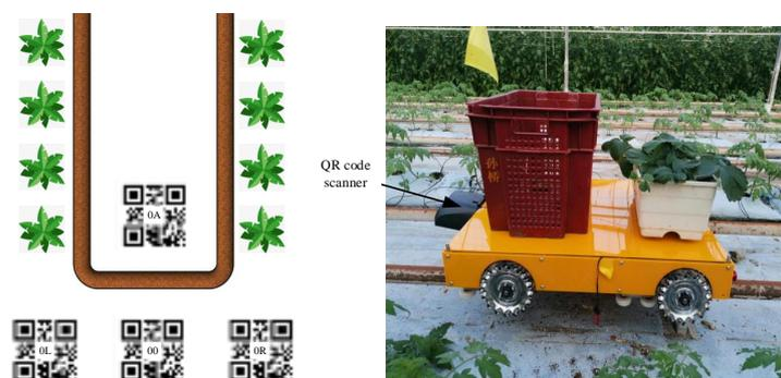
**Figure 3.** Diagram of the two-dimensional code localization.
