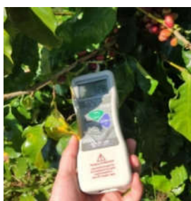
Figure 10. Tensile test using a digital push-pull meter.
