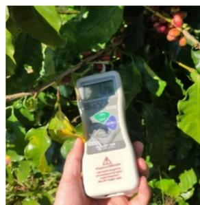
Figure 10. Tensile test using a digital push-pull meter.
