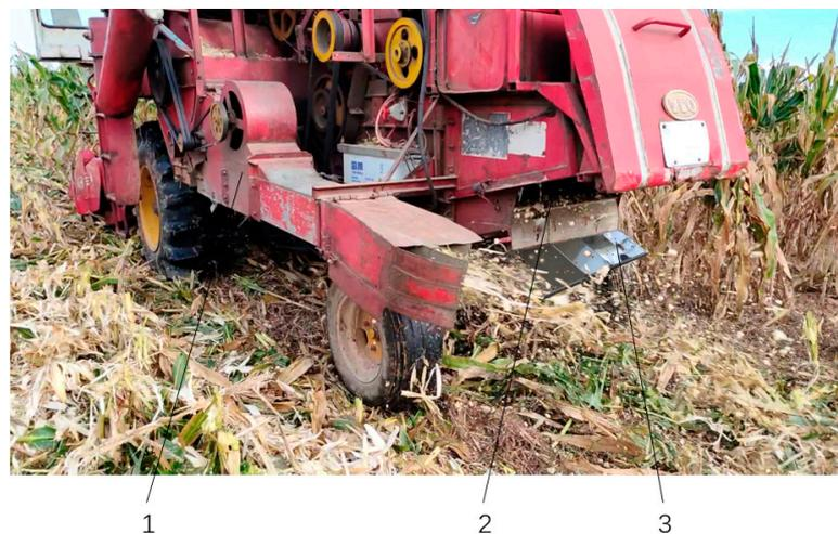
**Figure 12.** Field test: 1—LEVO GE40 harvester; 2—Cleaning miscellaneous mouth; 3—Loss monitoring sensor.
