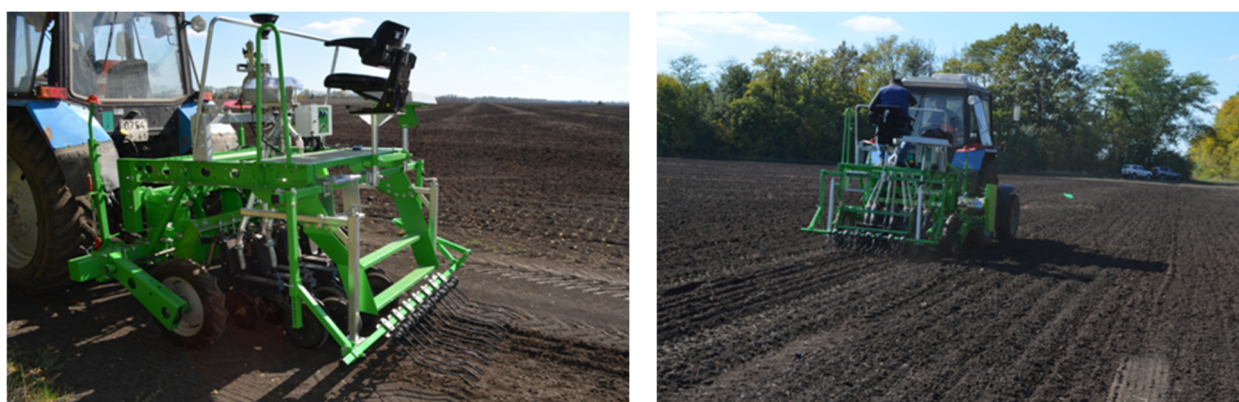
Figure 3. Trititrigia sowing with the Demetra seeder.
