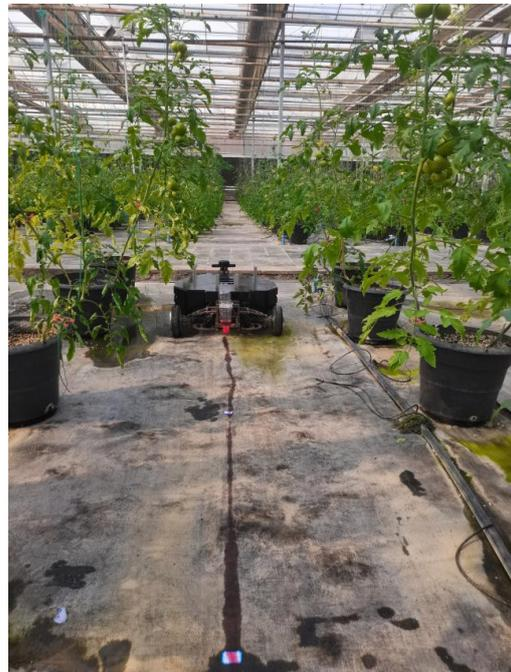
**Figure 25.** Experiment scene of setpoint parking in the greenhouse tomato growing area.
