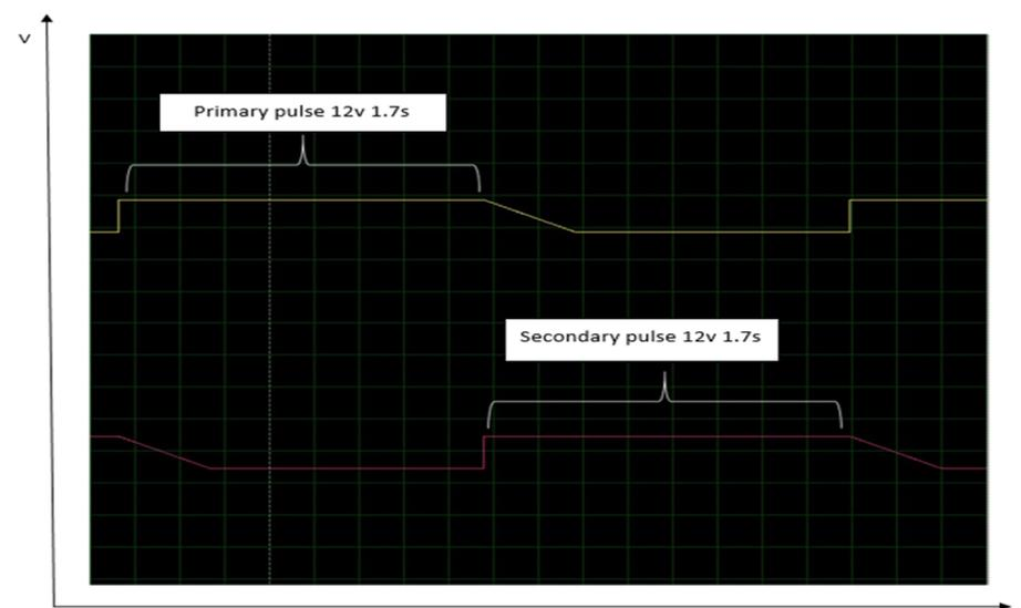
**Figure 11.** Test reading for electric brake pulse on a 12 v scale per square and 2 s.
