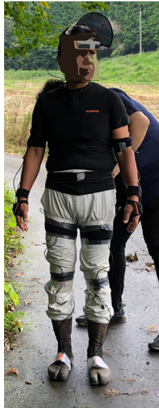
Figure 2. Subject equipped with the motion capture device Xsens MVN.
