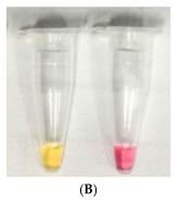
**Figure 1.** (**A**) Overview of the 3D-printed portable thermal block device. The plastic box contains a heating metal block, set to operate at 65 °C for 30 min. The device is powered by a portable power bank and connected via Bluetooth to a tablet. (**B**) The positive reaction (amplified DNA) is visualized by the color change from pink (negative signal) to yellow (positive signal).
