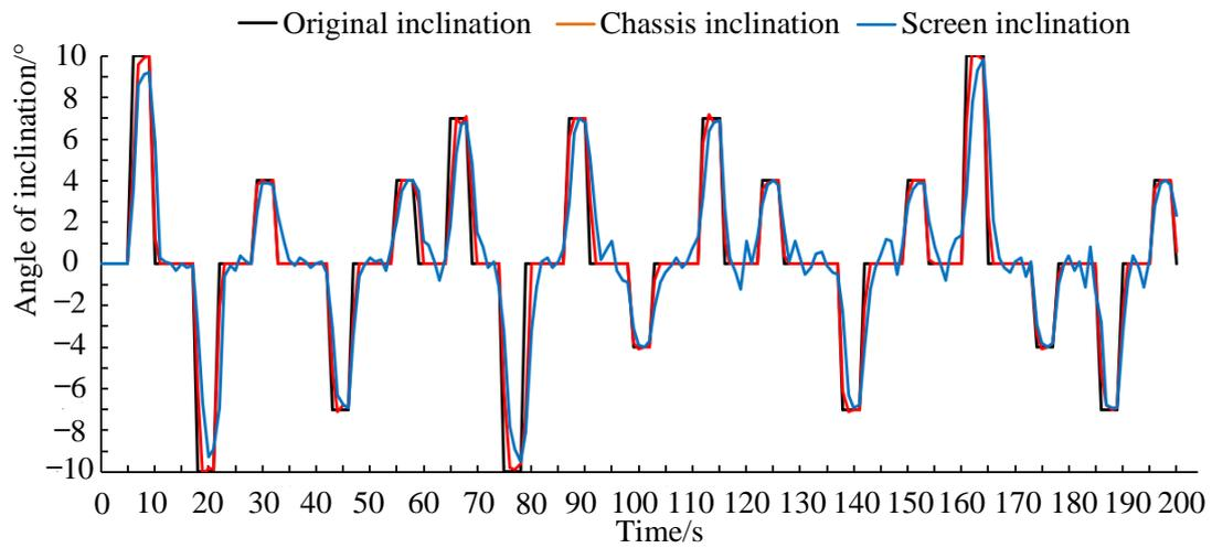
Figure 12. Pavement test results of tracking effect.
