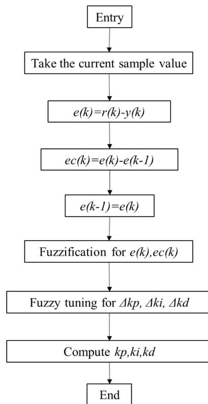
**Figure 7.** Workflow of the fuzzy PID controller.
