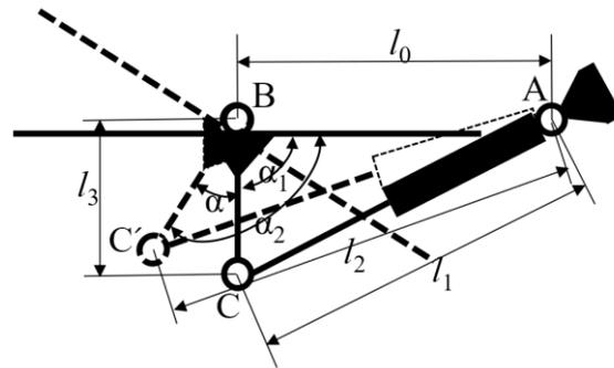
Figure 3. Simplified model of the screen-leveling mechanism.
