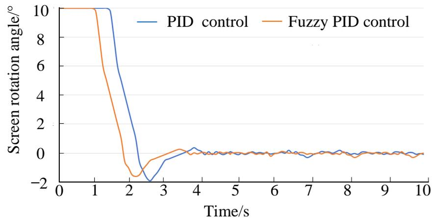
**Figure 11.** Comparison of PID and fuzzy PID.
