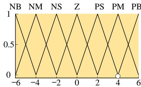
Figure 8. Input and output membership functions.
