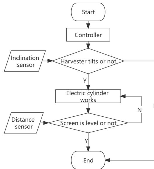
**Figure 2.** Working principle of the automatic leveling control system for cleaning the vibrating screen.
