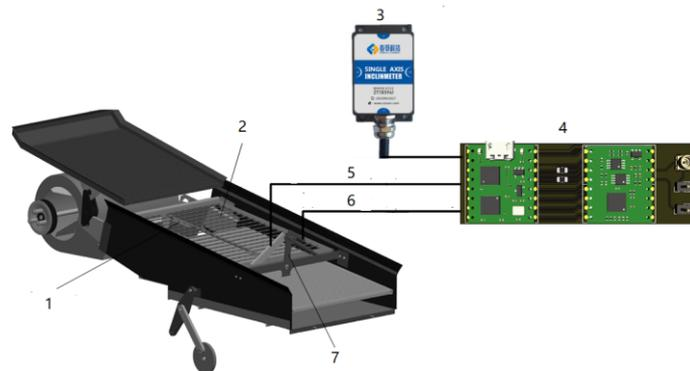
**Figure 1.** Structural composition of automatic leveling system. 1: rotating shaft; 2: screen; 3: inclination sensor; 4: controller; 5: distance sensor; 6: electric cylinder; 7: swing rod.
