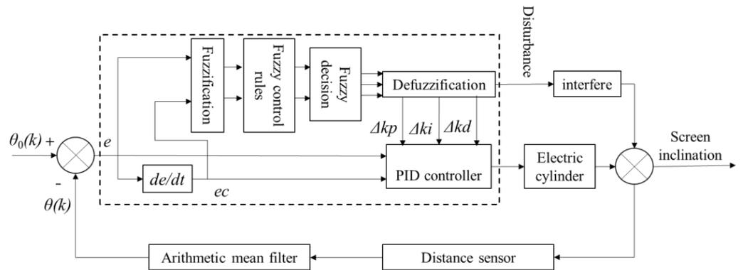
Figure 6. Structure of the fuzzy PID controller.
