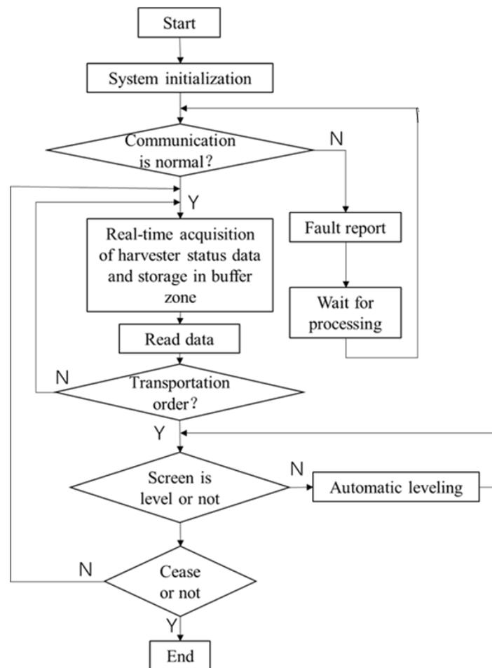
**Figure 4.** Main program control flow chart.
