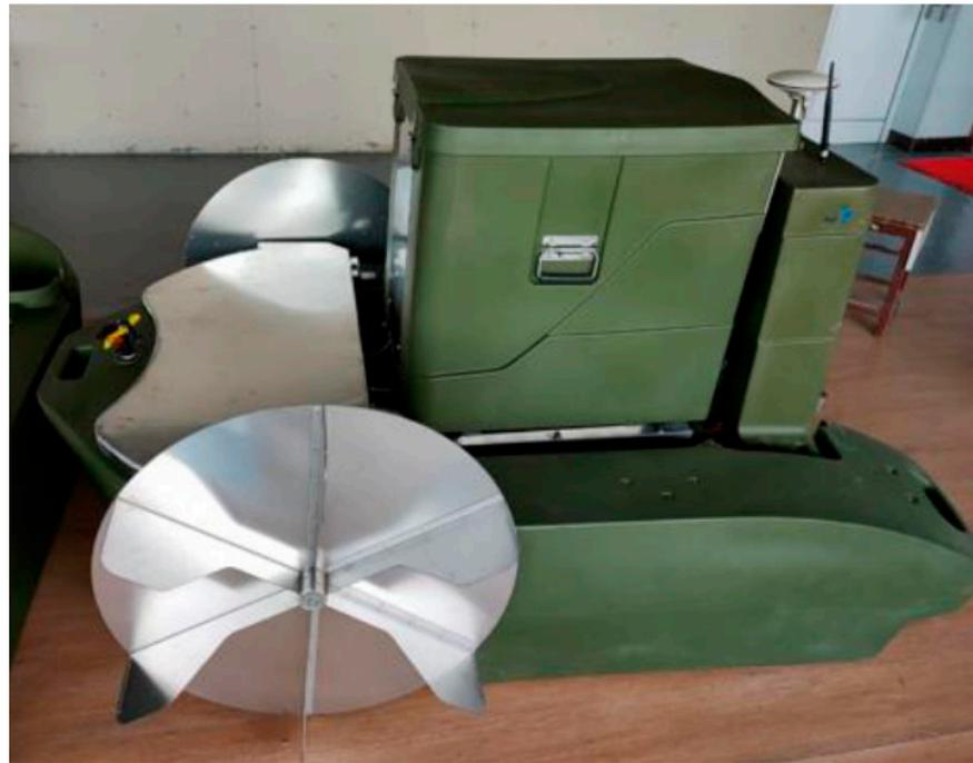
**Figure 4.** Prototype of automatic baiting device.
