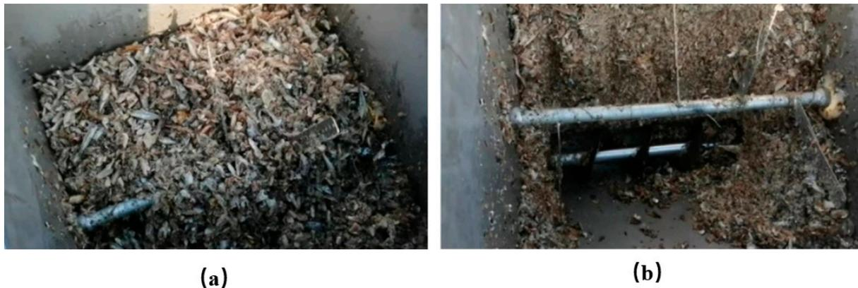
**Figure 13.** Experimental results of the baiting device with the agitation device installed: (a) the state of bait distribution at the beginning of the experiment; and (b) bait distribution status at the end of the experiment.
